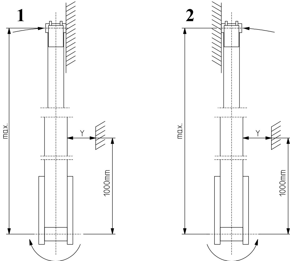
3. Measure the distance Y from the boom surface 1 at a distance of 1 m from the joint to be measured and note the result (refer to drawing).
