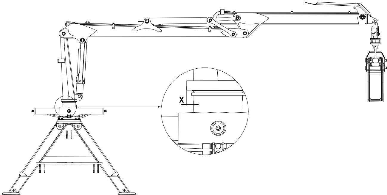
2. Measure the distance  $X$  from the flange surface 1 to the outer surface of the slew housing 2. Note the result (refer to drawing).
