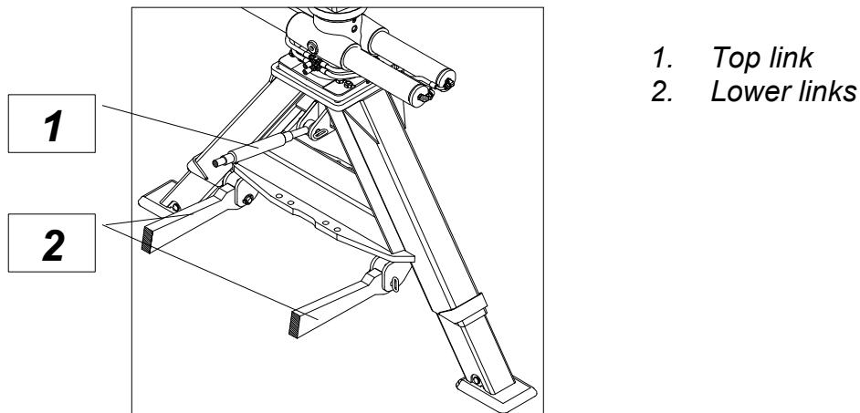
Only use the tractor's three-point hitch to transfer the loader. Never use the loader to lift anything when it is attached to the hitch, as this may damage the hitch or the loader frame and tilt the loader.
