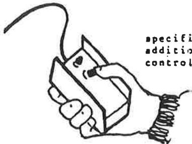
**EXTRA CONTROL PANEL:** The Igland 6000/2LH in standard specification is equipped with 2 plugs and control panel. An additional control panel with 5m cable allows the winch to be controlled from both outside and inside the cab.
